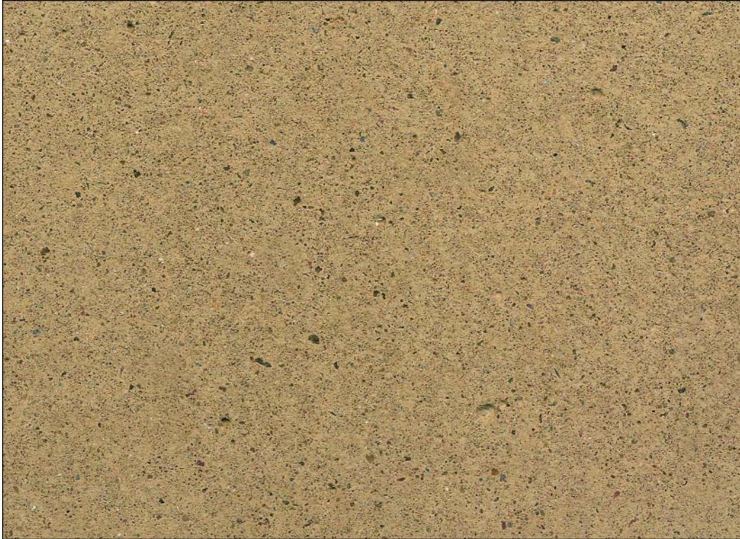
CPCI 171 rustic brown stone 25%, red granite 75%, Shaws red sand, white cement, tan pigment, light sandblast
