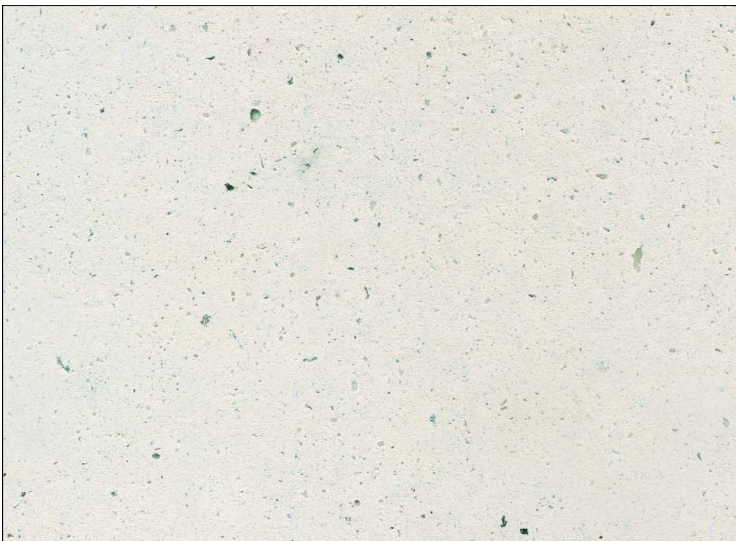
CPCI 107 75% calcite, 25% northern pink granite, white sand, white cement, light sandblast
