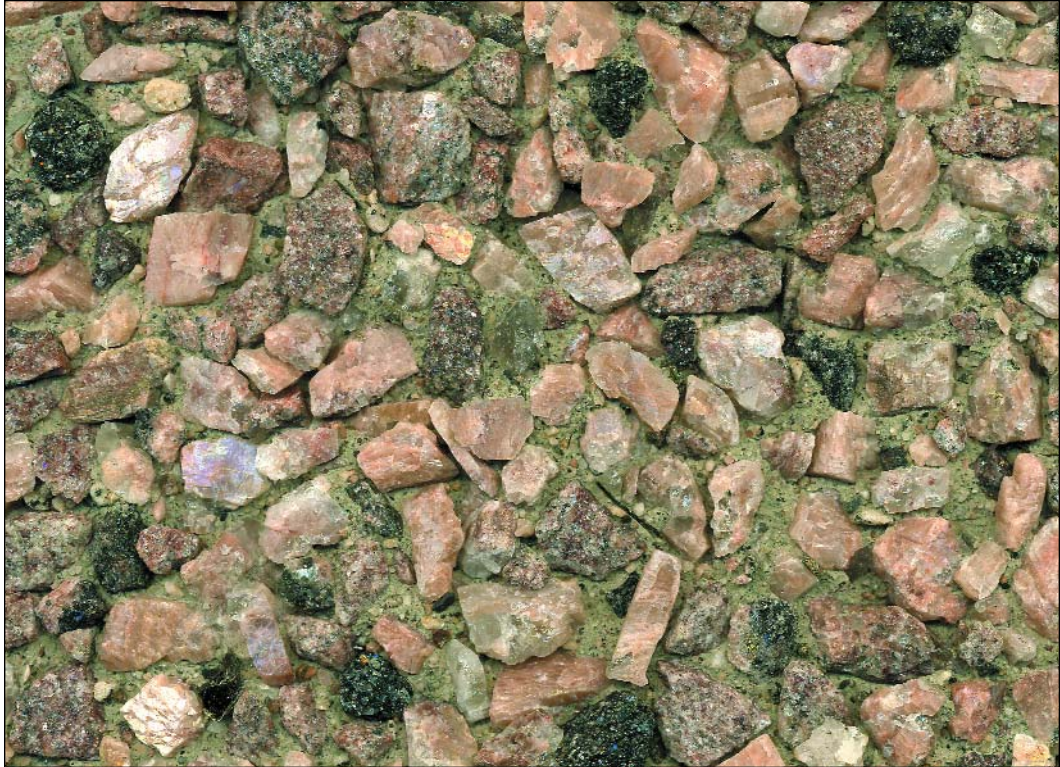
CPCI 154 northern pink granite, empire red granite, Ottawa red coarse sand, grey cement, exposed aggregate
