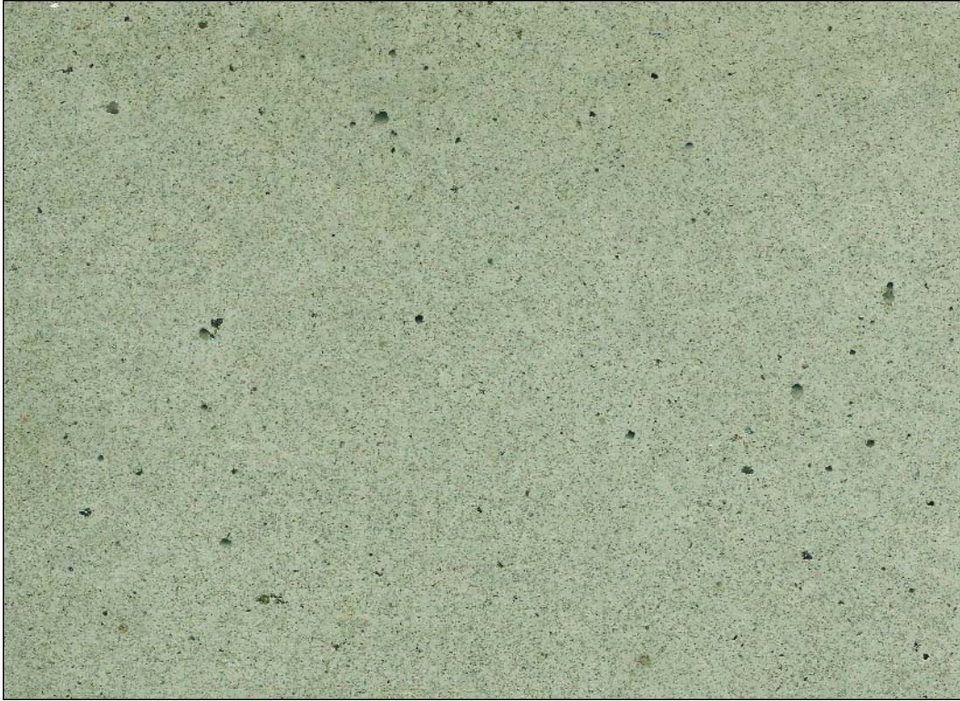
CPCI 151 northern pink granite, empire red granite, Ottawa red coarse sand, grey cement, light sandblast
