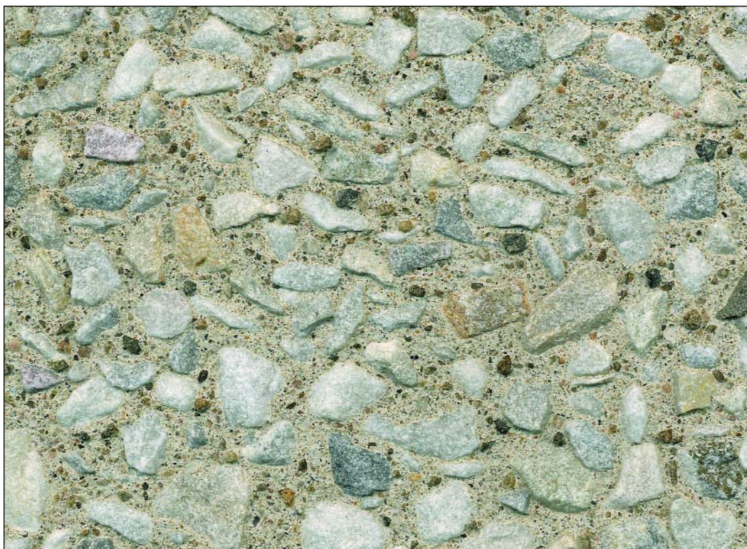
CPCI 148 \frac{3}{8} - \frac{5}{8} inch crushed white marble, natural brown sand, white cement, medium sandblast
