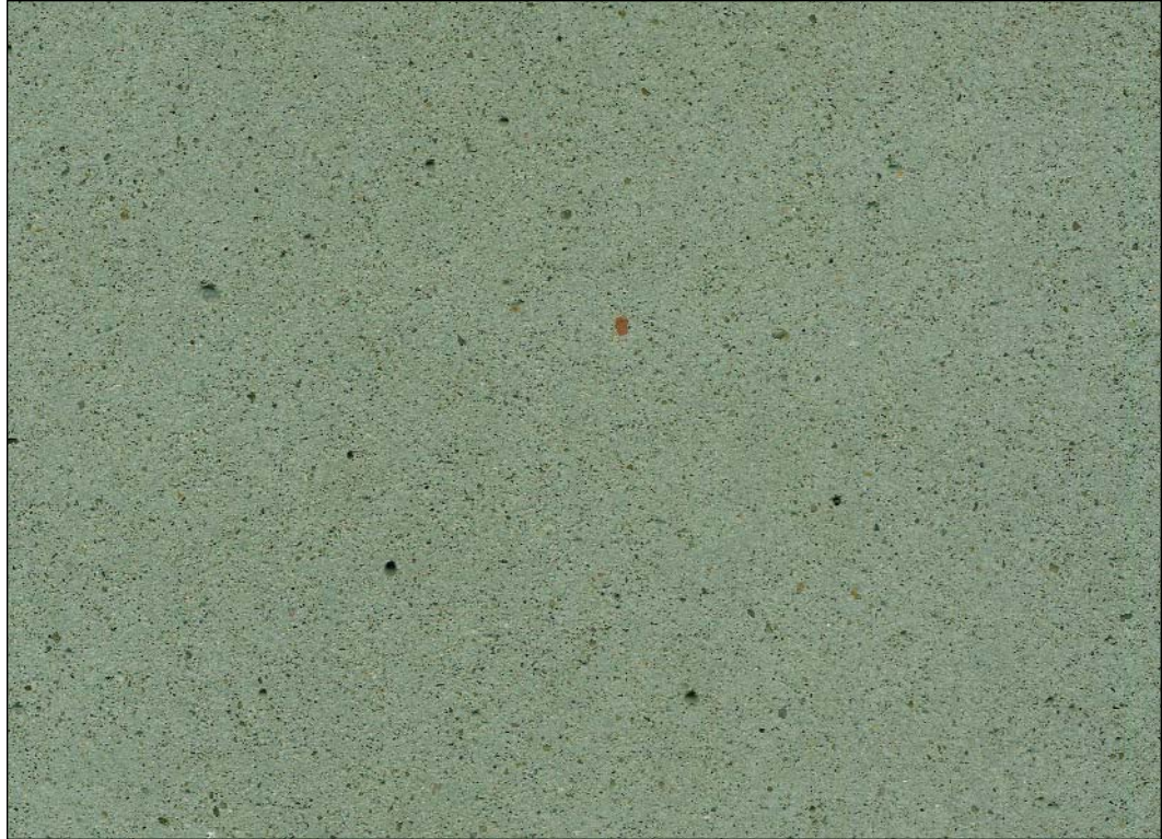
CPCI 165 natural multi coloured stone, Shaws red sand, grey cement, light sandblast
