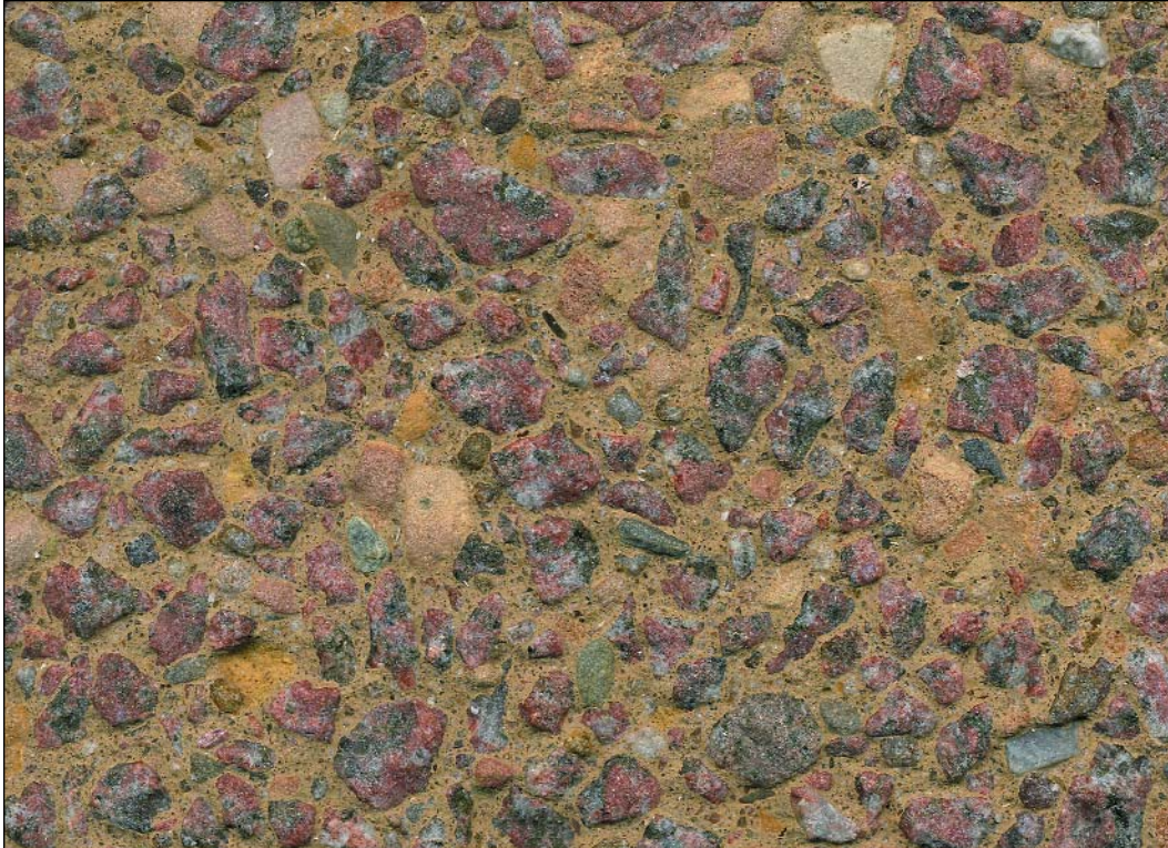
CPCI 172 rustic brown stone 25%, red granite 75%, Shaws red sand, white cement, tan pigment, very heavy sandblast
