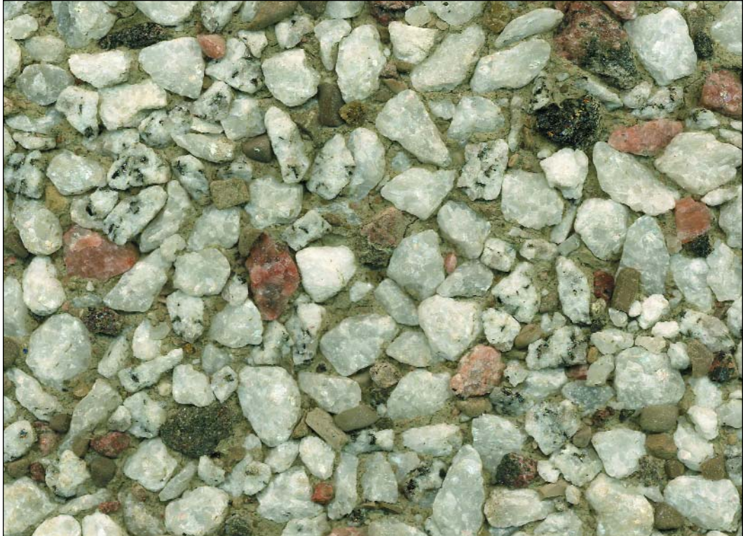
CPCI 110 calcite, light grey granite, empire red granite, northern pink granite, concrete sand, grey cement, exposed aggregate
