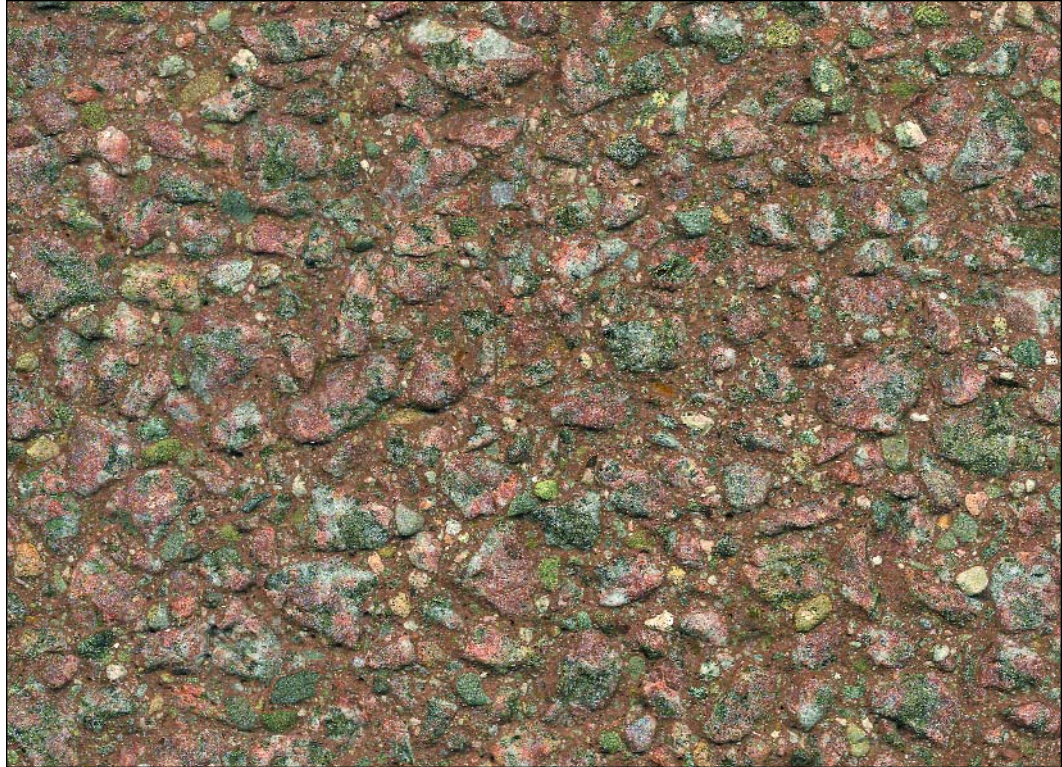
CPCI 174 red granite, natural concrete sand, grey cement, red pigment, heavy sandblast
