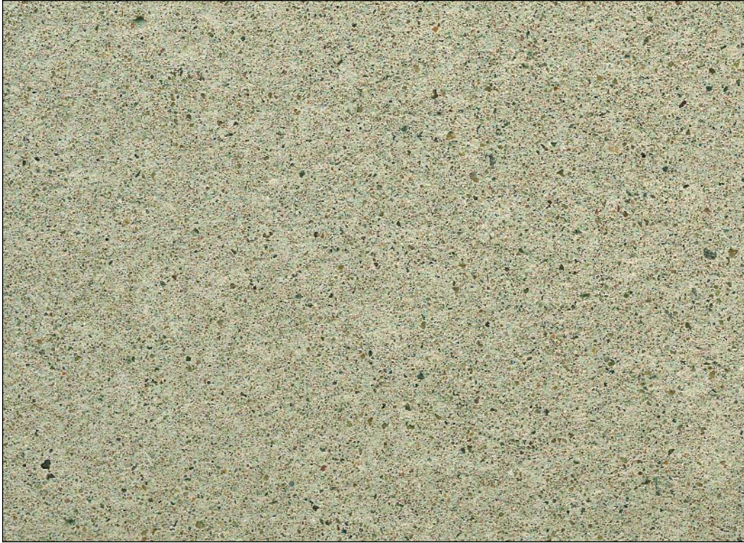
CPCI 163 red granite, Shaws red sand, 60% white cement, 40% grey cement, light sandblast
