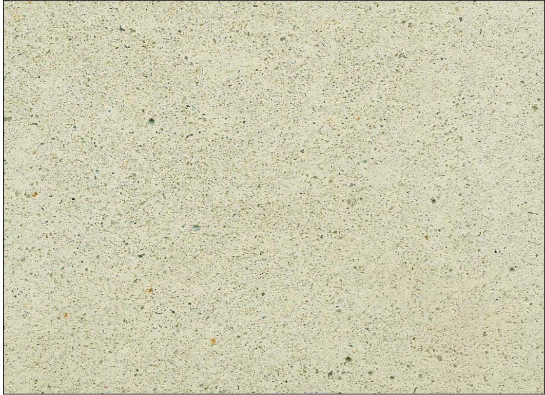
CPCI 133 grey limestone, white silica sand, white cement, tan pigment, light sandblast
