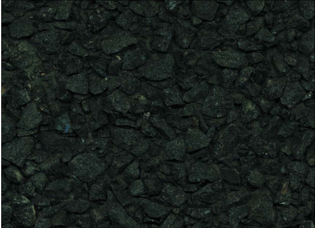
CPCI 170 black granite, < 1/4 inch black granite sand, grey cement, black pigment, exposed aggregate
