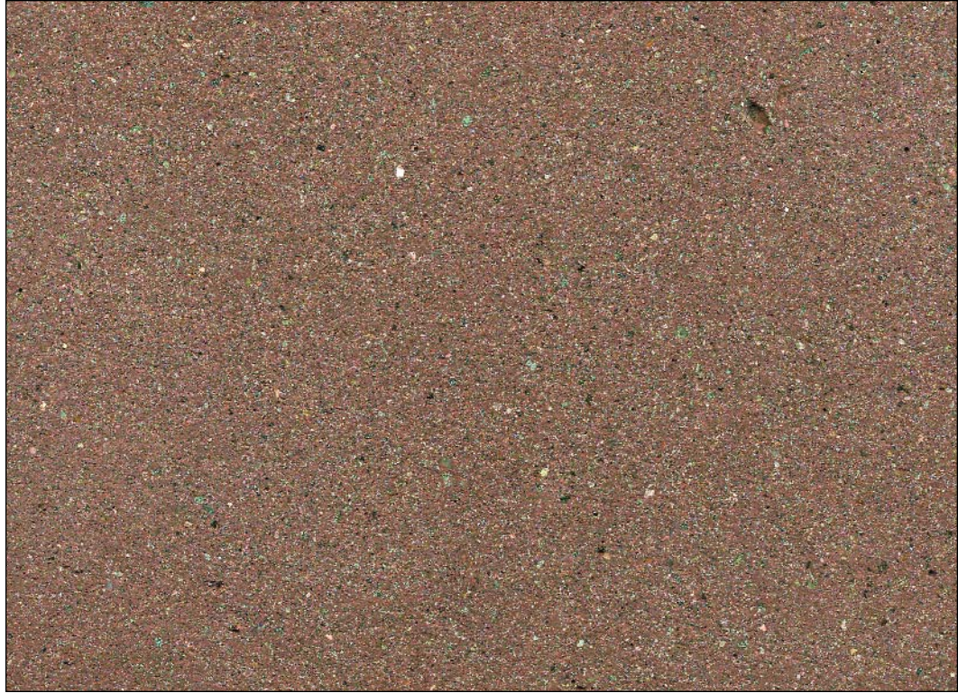
CPCI 173 red granite, natural concrete sand, grey cement, red pigment, light sandblast
