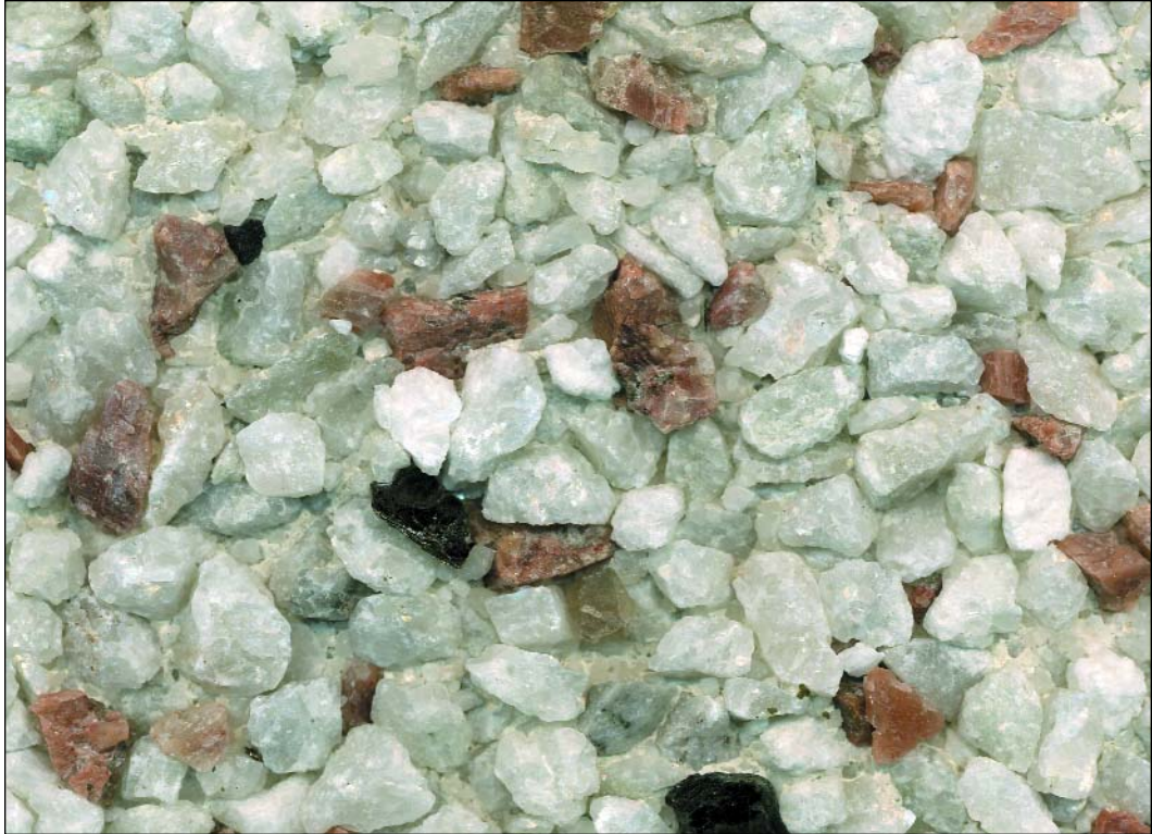
CPCI 109 75% calcite, 25% northern pink granite, white sand, white cement, exposed aggregate
