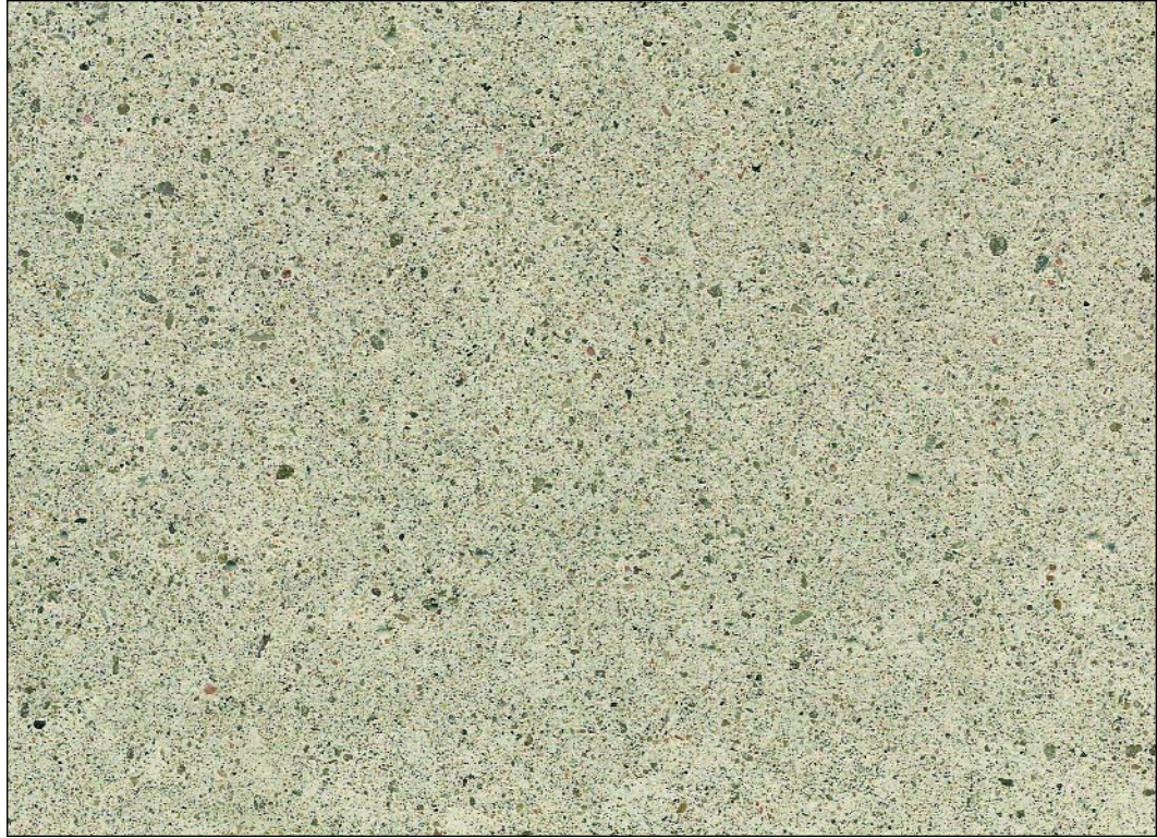
CPCI 149 limestone, concrete sand, white cement, light sandblast
