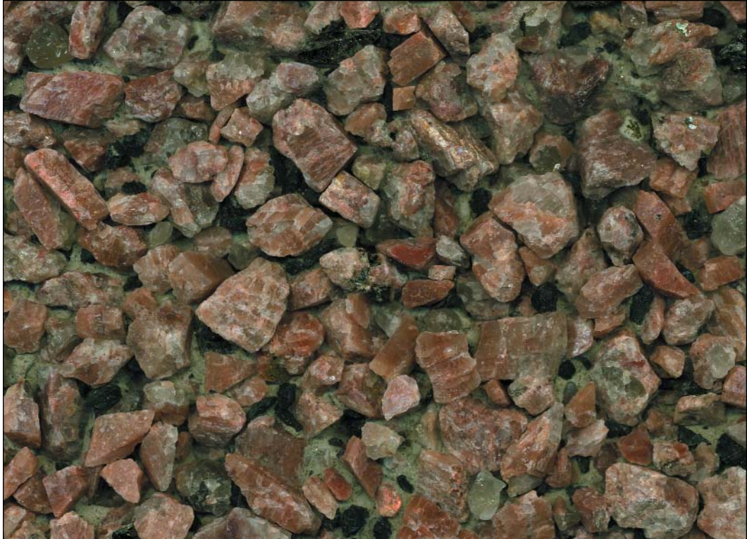
CPCI 158 northern pink granite, 1/4-3/8 inch black granite, brick sand, grey cement, exposed aggregate
