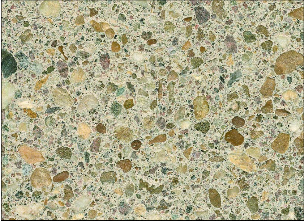
CPCI 137 Alabama brown river gravel, Ottawa red coarse sand, white cement, heavy sandbast
