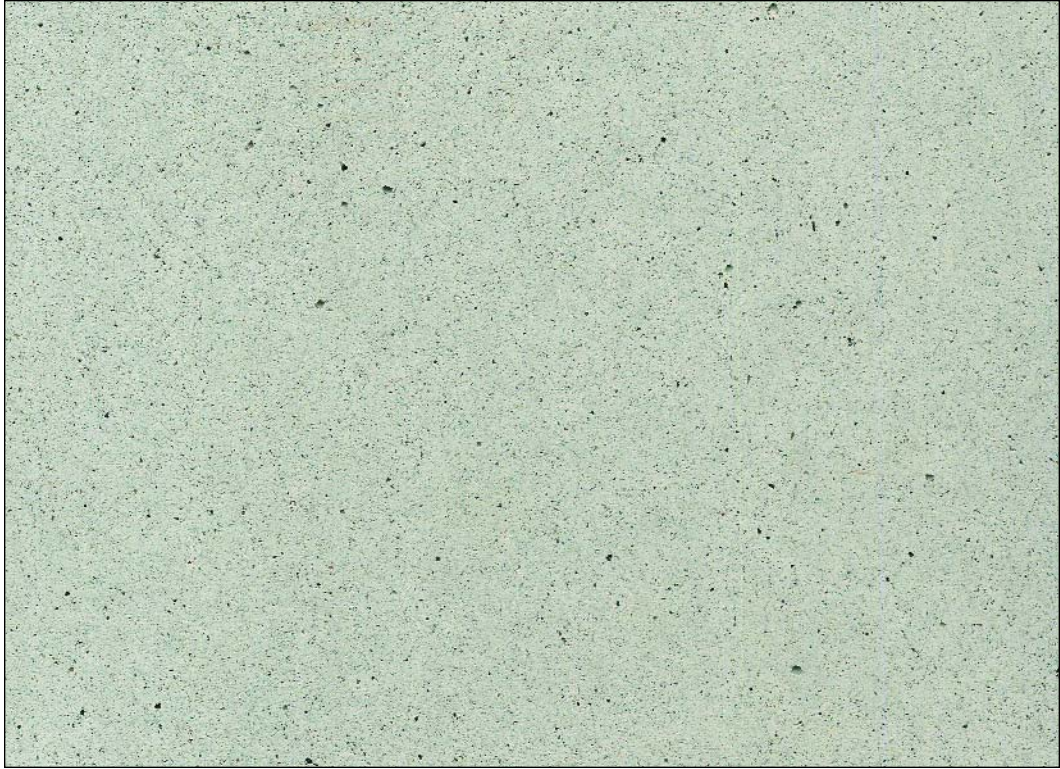
CPCI 161 limestone, Belmont rose granite, < ¼ inch black granite sand, Belmont rose granite sand, white cement, light sandblast
