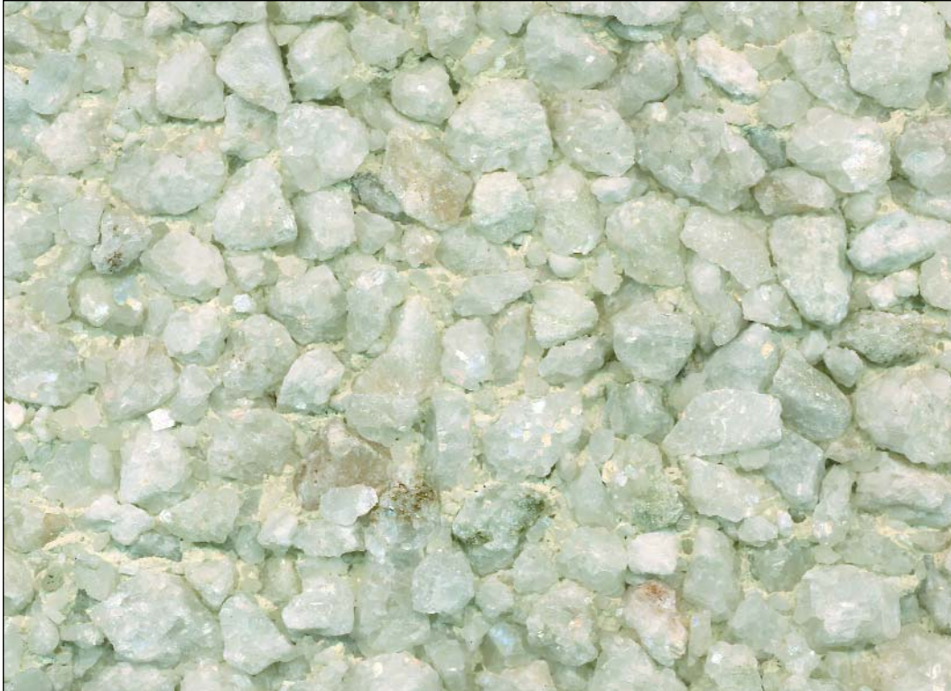
CPCI 104 calcite, white sand, white cement, exposed aggregate
