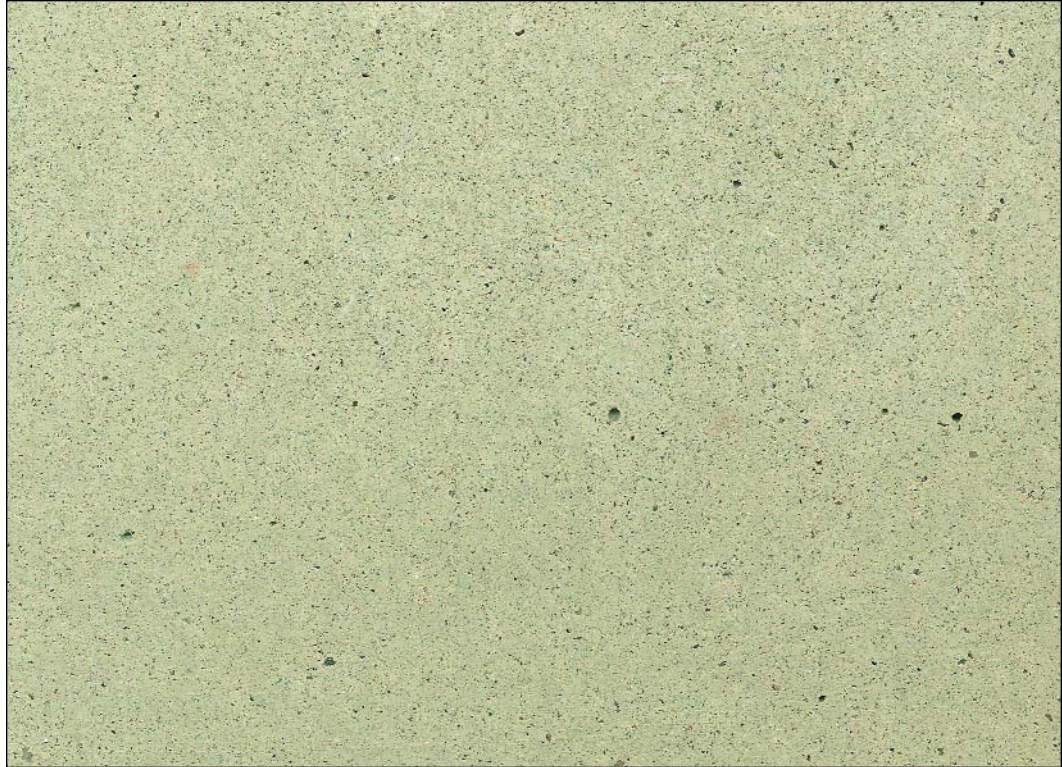
CPCI 129 Dufferin limestone, Ottawa red coarse sand, 70% white cement, 30% grey cement, light sandblast
