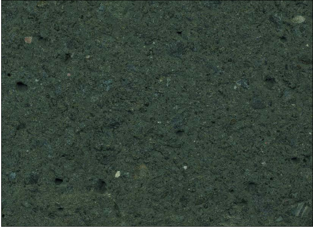
CPCI 169 black granite, < 1/4 inch black granite sand, grey cement, black pigment, medium sandblasted
