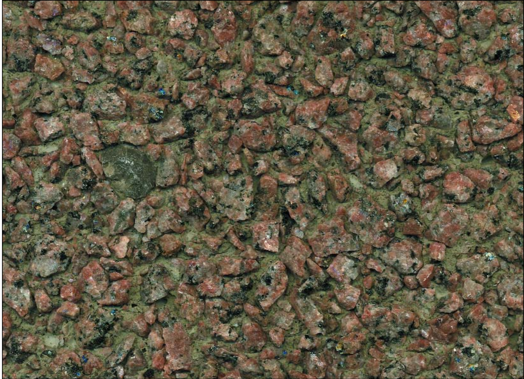
CPCI 157 Belmont rose granite, Belmont rose granite sand, grey cement, exposed aggregate
