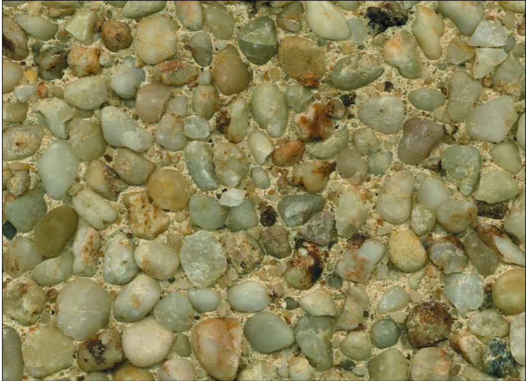
CPCI 138 Oriskany river gravel, 400 Bell sand, white cement, exposed
