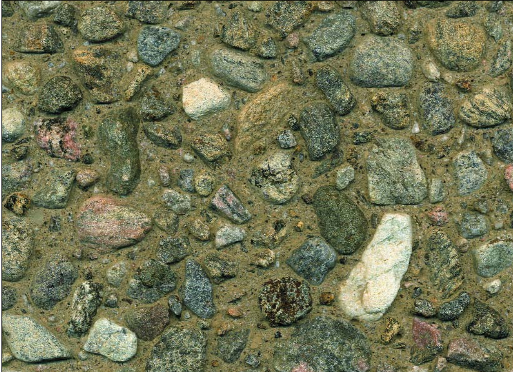
CPCI 140 \frac{3}{8} - \frac{5}{8} inch multicoloured river gravel, natural brown sand, grey cement, dark yellow pigment, medium sandblast
